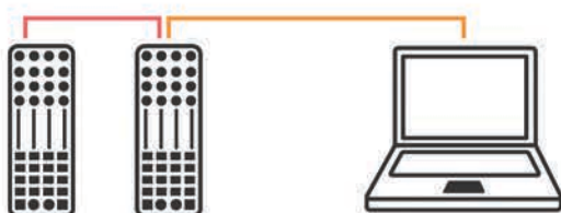
:K1 CONTROLLERS via X:LINK + LAPTOP via USB
