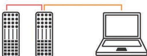
:K1 + :K2 CONTROLLERS via X:LINK + LAPTOP via USB
