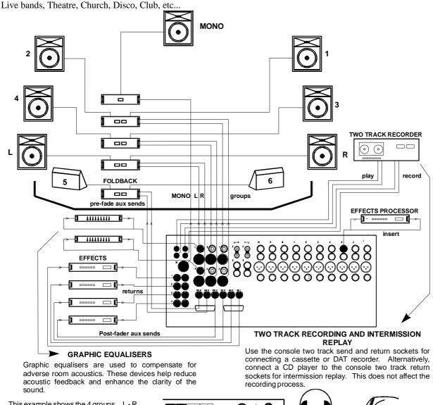
This example shows the 4 groups, L-R and Mono outputs feeding a 7 stack FOH amplification system. The groups provide independent control of the additional left and right loudspeaker stacks or may be used for zone feeds or for subgrouping to the L-R mix.
