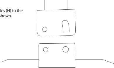
**4.** Now insert medium bolt (A) through the smaller holes and secure with washer (D) and nut (E).
