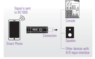
The On-Stage BC1000 allows you to stream audio wirelessly by picking up the signal from your Smart Phone and connecting it to a console, speaker or any other device with XLR input interface.
