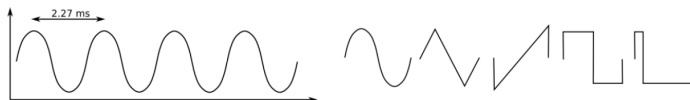
A single cycle of each waveform: sine, triangle, sawtooth, square, and pulse
