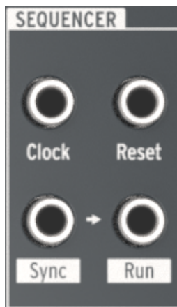
The Sequencer section of the patch bay
