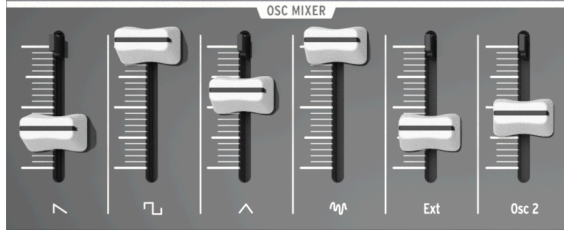
The Oscillator mixer section
