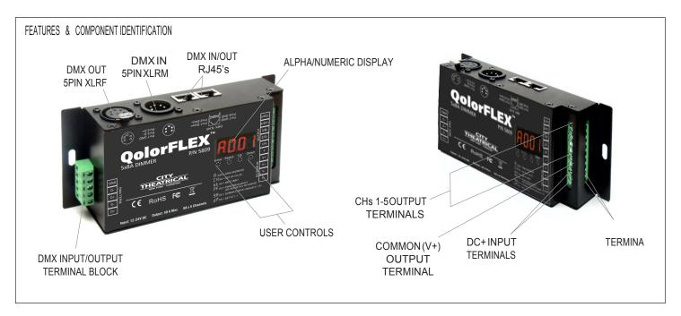
The QolorFLEX™ 5x8A Dimmer can control a full 40A of LED tape spread over five output channels of 8A each. This allows the control of unique combinations such as RGB tape (three channels) and bi-color tape (two channels), or RGBX tape (four channels) and a single color tape (one channel) together in one unit. The QolorFLEX 5x8A uses constant voltage technology which ensures consistent full range dimming that is especially important at low end light levels.
