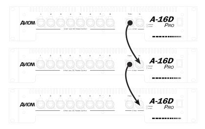
The example shows three A-16D Pro Distributors connected in a daisy chain. This provides twenty-four powered A-Net outputs. Any number of A-16D Pro Distributors can be connected to provide additional expansion by connecting the A-Net Thru jack to the next Distributor's A-Net In jack.
