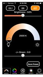
Start by creating a matrix of individual lights or groups of lights. Every light can be on one of 10 individual ZyLink channels with each control change affecting every fixture on that channel within each fixtures ability to do so.
