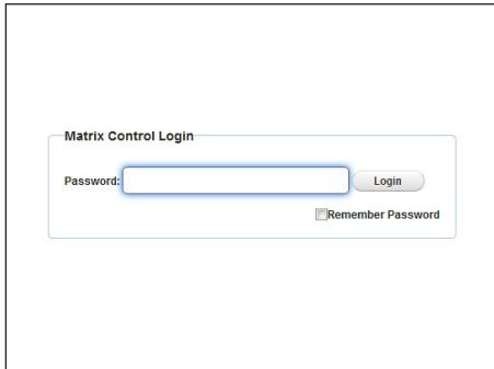
Open a web browser and go to the IP address of the DL-HDM88-FS. The default IP address is 192.168.0.178.
