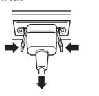
Unplug the connector pressing the two knobs.
