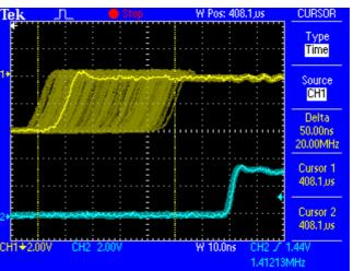
The screnshot shows an extremely jittery SPDIF signal of about 50 ns jitter (top graph, yellow). SteadyClock turns this signal into a clock with less than 2 ns jitter (lower graph, blue). The signal processed by SteadyClock is of course not only used internally, but also used to clock the digital outputs. Therefore the refreshed and jitter-cleaned signal can be used as reference clock without hesitation.
