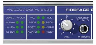
The red **HOST** LED lights up when the Fireface 800 has been switched on, thus signalling the presence of operating voltage. At the same time it operates as Error LED, in case the FireWire connection hasn't been initialised yet, or has been interrupted (Error, cable not connected etc.).
