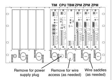
A 15-zone PCM system without talk-back capability, six-zone slave assembly mounted at left:
