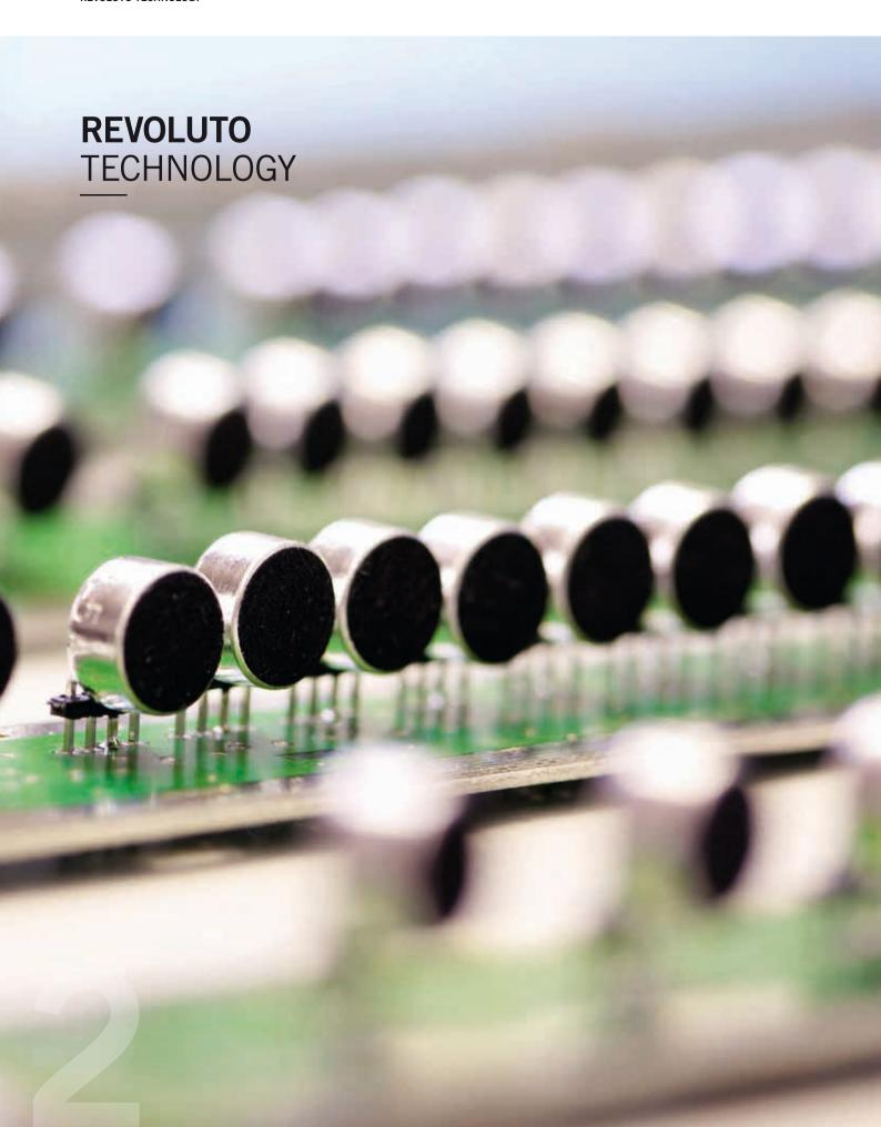
**The Revoluto principle** – The Revoluto principle is based on patented microphone array technology, where microphone capsules are arranged in either a horizontal or vertical row.
