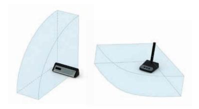
The horizontal and vertical arrangements of the microphone arrays differentiate in design as well as in the alignment of the corridor characteristic, which is displayed above. Depending on the request for design, room acoustics and sound reinforcement the appropriate variant can be selected to make optimal use of the advantages of the Revoluto technology.
