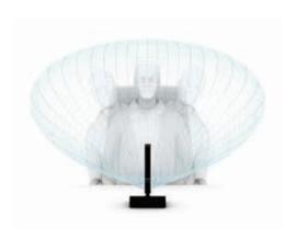
The vertical arrangement of the microphone array results in a horizontal corridor characteristic allowing maximum freedom of movement to the right and left without large volume fluctuations. The attenuation above and below the microphone limits the recording of signals and noises from the ceiling and table.
