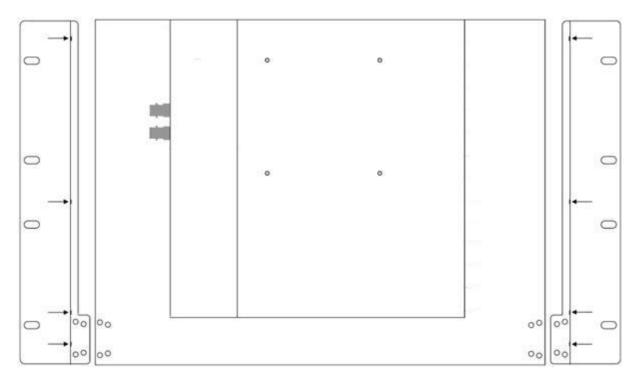
Use the supplied screws to attach the left and right rack ears. You will see there are four screws on either side, as illustrated above, plus additional screws at the base of each rack ear, as illustrated below.
