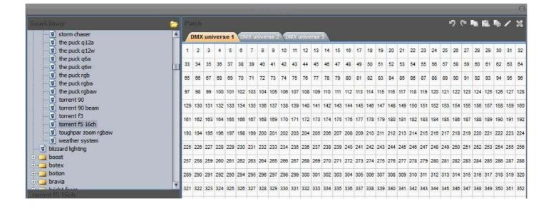
There are two ways to patch a fixture into the address map. The first is to drag and drop a particular profile from the list on the left into the address map. The second is to use the tools located at the bottom left-hand area of the Patch Manager window.
