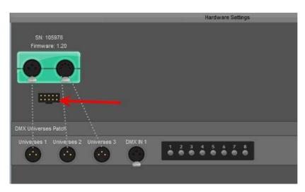
Plug you port panel to the HE10 interface port socket. Push some buttons to test your panel.
