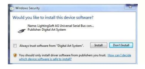
You are done! But remember, the software detects the USB interface when it starts. This means that you must have the USB interface connected to your computer before you open the control software. Otherwise, there will be no communication between the software and the interface.
