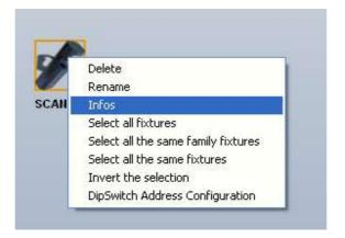
A window appears with the fixture's name, manufacturer's name, Type of fixture, number of channels, the address range and the number of fixtures for this icon.
