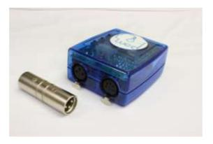
To convert the DMX input to an DMX output you need a DMX converter like the one pictured.
