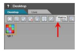
The matrix window appears. To select or deselect a fixture just click on the fixture icon, the blue color means that the fixture is selected. You can select all the fixtures at the same time by right clicking in the matrix window and choosing "Select All". Additionally, you can highlight individual rows and columns by right clicking on a cell in the row or column you wish to highlight and choosing either "Select row" or "Select col".
