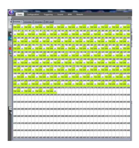
The DMX Level is in green, in this example the value is 127 for the address 234.
