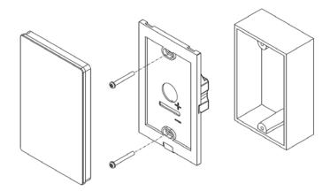
Designed to be installed within an installation grade junction box with an bolt spacing of **82.5mm** centre to centre.
