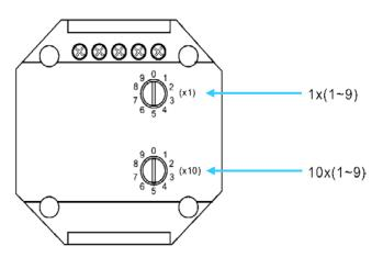
Set the starting address "X" on rear using the rotary encoders to a value between 0 and 63 using both the (10x) and (1x).
