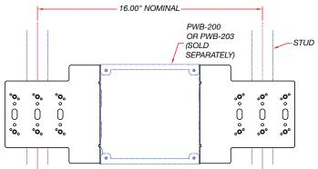
THE PWB-20X-MNT IS A SET OF BRACKET EARS THAT ALLOW THE INSTALLER TO POSITION THE PWB-200 OR PWB-203 AT DIFFERENT LOCATIONS BETWEEN THE STUDS WHILE MOUNTING.
