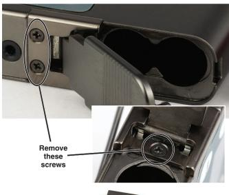
Save the door assembly parts for re-installation later
