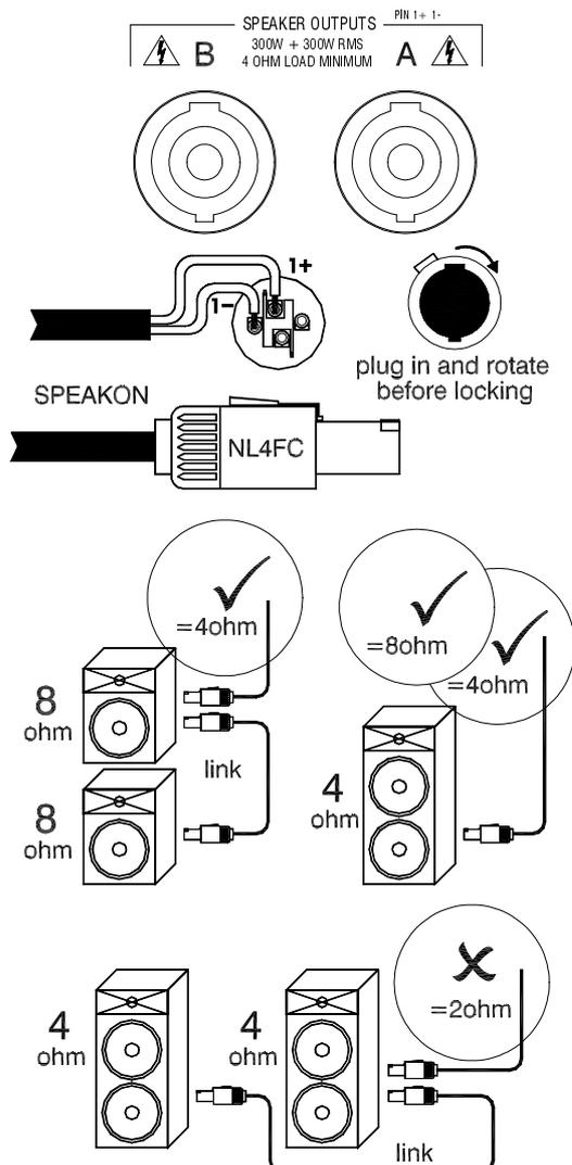
The power amplifier loudspeaker outputs are available on industry standard locking Speakon® connectors. Use the MODE function to determine which console mix is routed to these outputs. The outputs can be configured as shown above.
