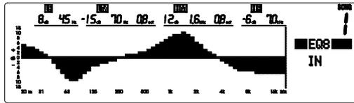
The LF band can become a sweepable 12dB per octave high pass filter (HPF) to cut low frequencies. This is useful in eliminating the low ‘popping’ sound associated with close vocal miking or to cut out low frequency noise. Simply turn the LF gain control to minimum and adjust the frequency control for the required cut off point.
