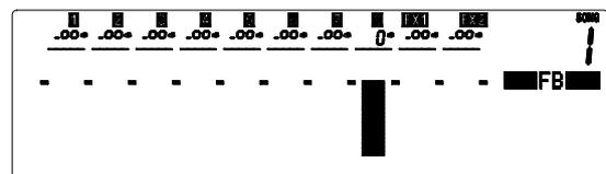
The soft strip becomes the foldback send controls, one for each channel. The normal operating level is 0dB but 6dB of gain is available if required. Press RESET to turn all the sends off. Press UNDO to restore the last settings or those marked by pressing ENTER.
