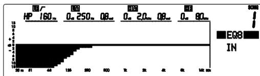
Press the OUT key to switch the EQ in or out. Press RESET to instantly reset the EQ flat. You can copy the EQ settings to another channel by pressing the COPY key. The PASTE key will illuminate. Select a different EQ, press PASTE to see the copied settings instantly take effect. The PASTE key remains lit to tell you that valid copy data is available until you select an unrelated screen or switch the console off.
