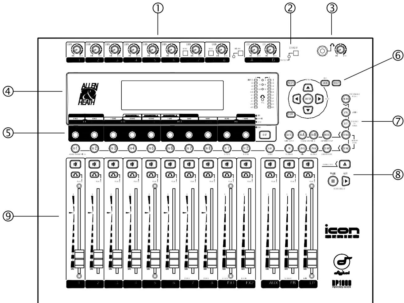
The DP1000 and the DL1000 front panel control layout is the same except for the labelling of the A, B level controls and MODE select key. This is because the DP1000 includes a built-in power amplifier, while the DL1000 provides balanced XLR outputs instead. The controls are soft touch for user comfort, and the display and keys are backlit for viewing in dark conditions.
