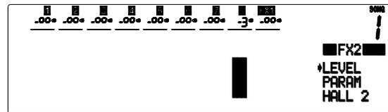
The soft strip becomes the effects send controls, one for each channel. This sends the signal to the internal effects processor where the reverb effect is created. The ‘wet’ reverb signal is returned via the FX2 fader channel and added to the ‘dry’ signal routed directly to the mix.
