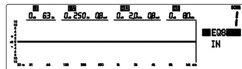
The soft strip beneath the display becomes the gain, frequency and width controls together with an illuminated in/out switch. Adjust these controls to experiment with the effect of boosting or cutting selected frequencies.
