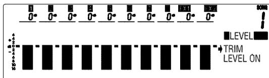
The soft strip provides a level trim control for each channel. The current settings are displayed as level bars with normal 0 position shown.
