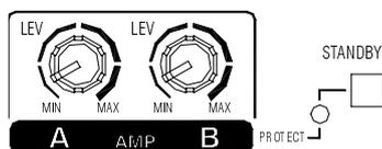
Press this switch to put the console into standby mode. This disconnects the loudspeakers using relays (DP1000 only), turns off (mutes) all the outputs, and locks the controls. The sound of the relays switching can be heard when the switch is pressed. Standby should be used when the console is left unattended to prevent the settings being tampered with, when equipment is plugged in or out, and when the system configuration is changed.
