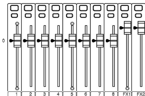
To recall the levels during live performance adjust and leave the faders at their '0' position. You can use the faders to make overall adjustments during the performance if required. If you do not want to use the stored trims turn them off as described above.
