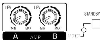
Press this switch to put the console into standby mode. This disconnects the loudspeakers using relays (DP1000 only), turns off (mutes) all the outputs, and locks the controls. The sound of the relays switching can be heard when the switch is pressed. Standby should be used when the console is left unattended to prevent the settings being tampered with, when equipment is plugged in or out, and when the system configuration is changed.
