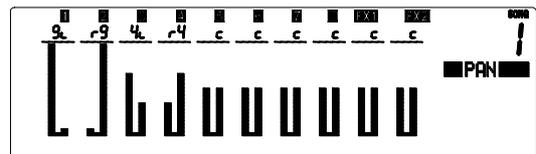
The 'soft strip' of rotary controls beneath the display becomes the row of PAN controls, one for each channel. Adjust these to balance the signal between left and right mix. Press RESET to set them all to centre image.
