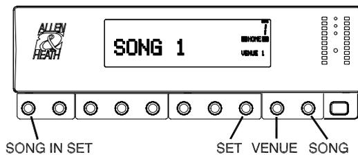
Use the soft strip control 7 to scroll through and select the **SET** you wish to perform. Press the flashing ENTER key to confirm, UNDO to escape.
