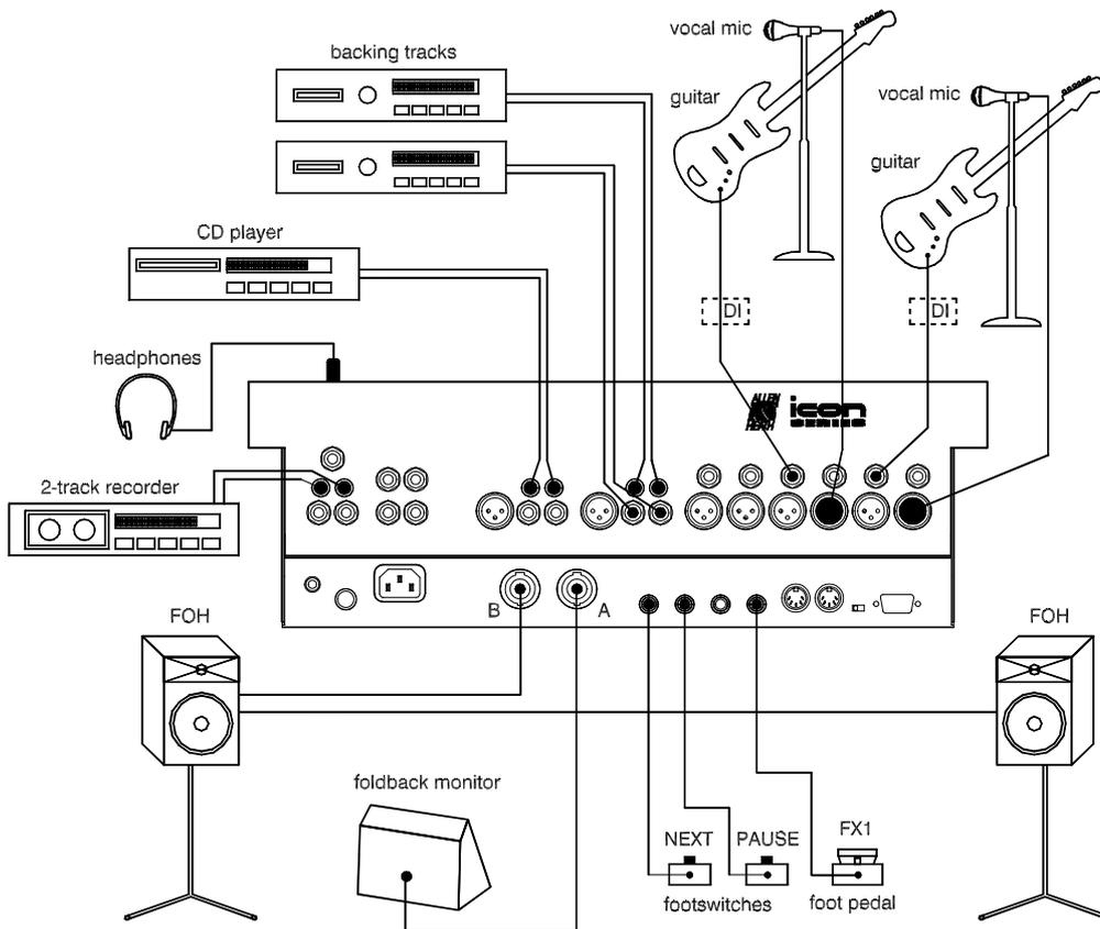
This setup is typical of a musical duo performing at a small venue such as a club or restaurant. No external amplifiers or signal processors are required. The musicians simply plug in the sources and loudspeakers, and use foot controllers to step through their pre-programmed performance.
