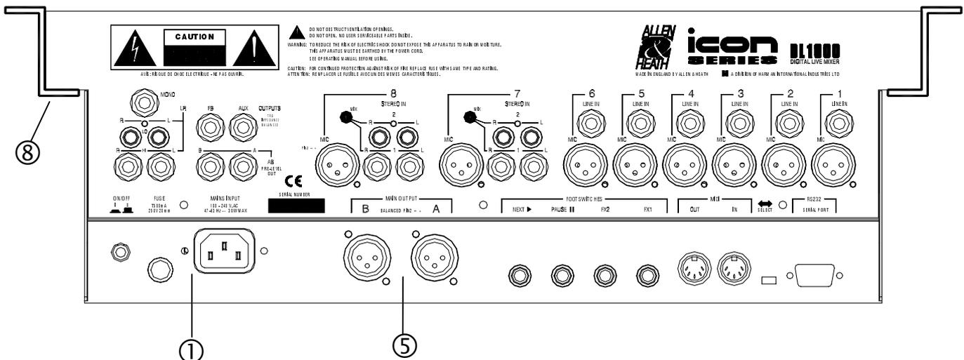
The DP1000 and the DL1000 rear connector panel layout is the same except for the **A AND B OUTPUTS** ⑤ and the **MAINS POWER INPUT** ①. The DP1000 has a pair of Speakon® connectors for the amplifier outputs and a country dependent power input, while the DL1000 has a pair of XLR connectors for the balanced line outputs and a universal power input.
