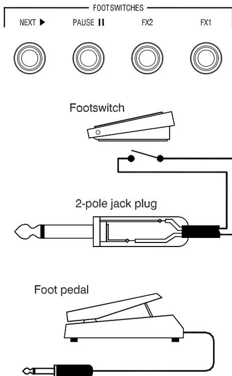
Up to four footswitches may be plugged in. Use standard 'passive' single pole footswitches wired to mono jack plugs. These are available from most musical equipment shops.
