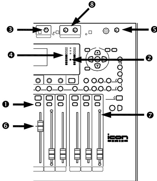
Press PFL ❶. The key illuminates red and the PFL active indicator ❷ lights to show that the meters now read the selected channel pre fader signal.
