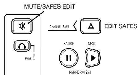
The SAFE key flashes to warn you that the mutes now edit the channel safes. Press a MUTE key to isolate the channel. The mute key flashes if the channel is made safe in this way.. Press again to restore the channel to normal operation. Press the flashing SAFE key to return to normal console operation. The SAFE key remains illuminated if one or more channels have been made safe.
