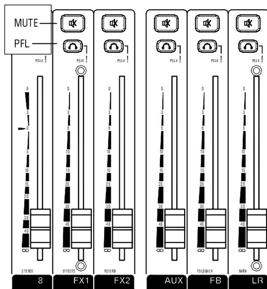
Each input, effect and output channel has an identical strip of controls. These are used during performance to check and control the signal levels to create the required mix balance and output level.
