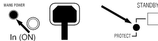
The DP1000 powers up in **PROTECT MODE** for two seconds. During this time the PROTECT indicator lights to show that the loudspeakers are isolated from switch on thumps, the fan blows at full speed to test the heat management system, the keypad and meters flash, and a start-up screen is displayed. After two seconds the indicator turns off, the relay clicks are heard as the loudspeakers are connected to the amplifiers, the fan slows to idle speed, and the HOME screen is displayed.
