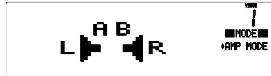
Press the MODE key. Press the ◀▶ keys to scroll through the three options. Press the flashing ENTER key to accept the change, UNDO to escape. Press RESET to restore the default LR setting.
