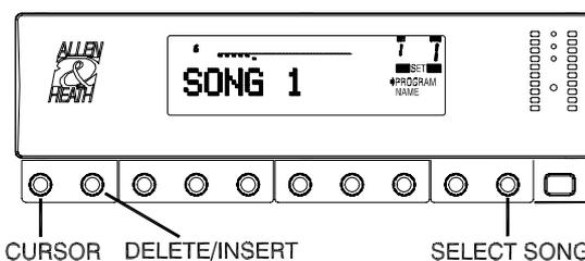
Select and confirm the set number you wish to program using the soft strip control 8. Use the cursor control 1 and song select control 10 to add songs to the set. Use control 2 to delete or insert songs at any point within the set. Scroll to the required point using the cursor control 1. Press ENTER to confirm your action, UNDO to escape. Press RESET to clear the set. You can COPY and PASTE programs from one set to another.
