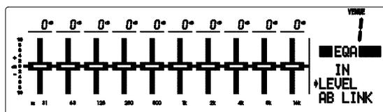
This divides the frequency range into ten bands which can be independently boosted or cut using the soft strip controls. This is used to adjust for room or loudspeaker acoustics. Press OUT to switch the EQ out, and RESET to instantly set it flat. EQ A and B can be linked using the AB LINK menu option for stereo operation.
