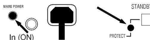
The DP1000 powers up in **PROTECT MODE** for two seconds. During this time the PROTECT indicator lights to show that the loudspeakers are isolated from switch on thumps, the fan blows at full speed to test the heat management system, the keypad and meters flash, and a start-up screen is displayed. After two seconds the indicator turns off, the relay clicks are heard as the loudspeakers are connected to the amplifiers, the fan slows to idle speed, and the HOME screen is displayed.
