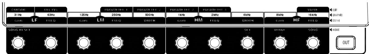
The row of 10 rotary controls together with the OUT key is known as the ‘soft strip’. This is because the function of these controls changes depending on the select key pressed. This means that only one set of controls is needed so simplifying the layout and preventing clutter. The functions are identified from the labels printed above or the number keys below. The OUT key is used to switch the selected EQ in or out of circuit.
