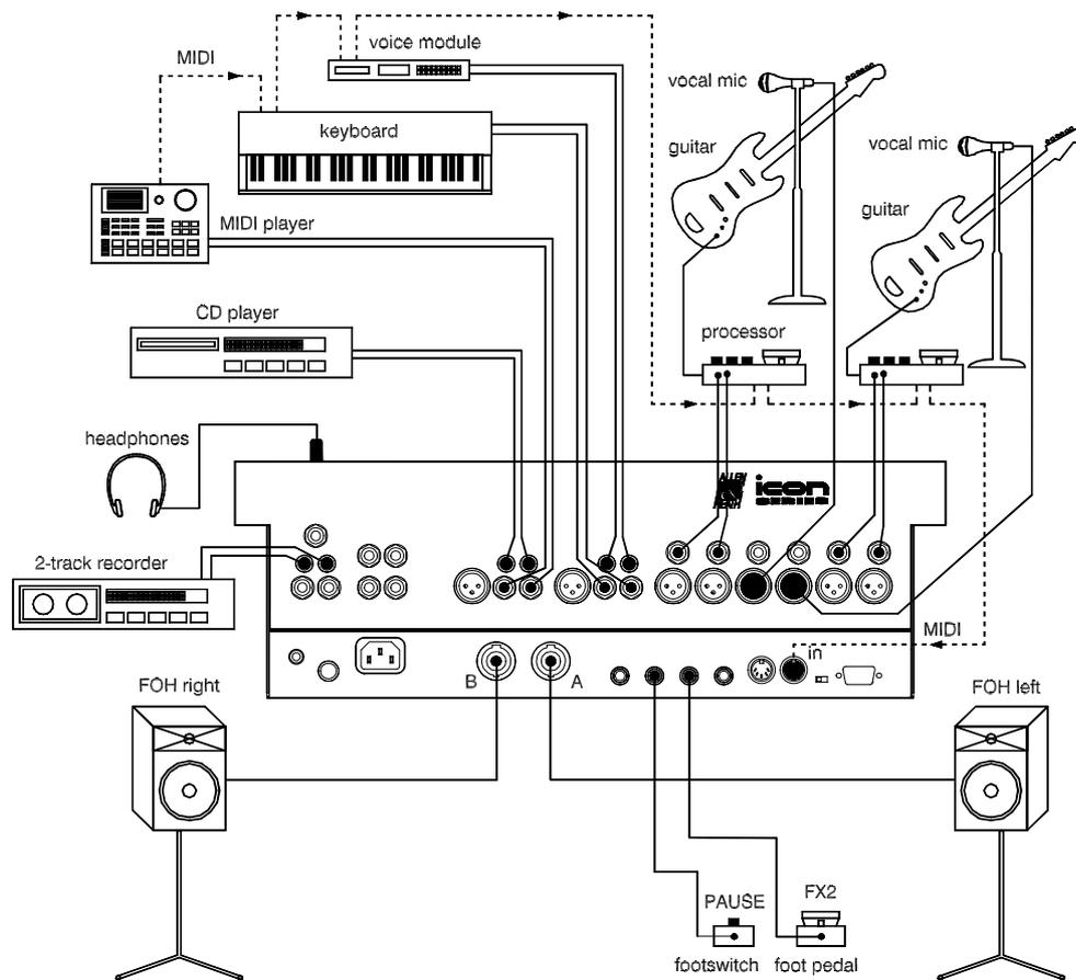
In this example three musicians perform using a sophisticated MIDI based stereo system without monitors, typical of many small venues. The sources and built in effects combine to produce a full stereo sound. The output AB mode is configured for L-R.
