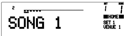
The selected set number and name are displayed together with a progress bar which shows you the number of song memories in the set and how far you have progressed. A small number indicates the current position in the set. Press the NEXT ► key or footswitch to advance to the next song. This recalls the memory instantly and without confirmation. The progress bar moves ahead and the new song name is displayed.
