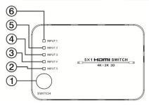
Front Panel: ①③HDMI input port, connect with DVD, PS3,Set-top Box and Note Book with HDMI cable ②HDMI output port, connect with HDTV or monitor with HDMI cable
