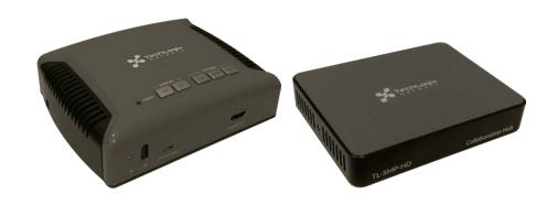
The TechLogix TL-SMP-HD is an HDMI collaboration system which includes a control system to turn on and off the display and adjust the volume on the display with physical buttons on the top of the transmitter. The display may be controlled by CEC or IR commands. EDID information from the display is passed to the HDMI input, which supports video signals up to 4K/30.
