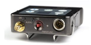
The housing is constructed of solid machined aluminum for lasting ruggedness. The exterior is finished with an ultra hard, black electroless nickel finish called *ebENi*.
