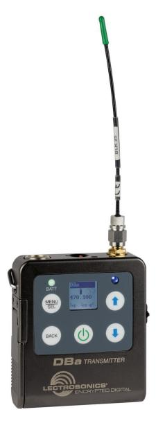
The DBa transmitter is a second generation design with specially developed, high efficiency digital circuitry for extended operating time on two AA batteries. The transmitter can tune in coarse or fine steps across the UHF television band from 470.100 to 691.175 MHz, with an output power of 50 mW. The pure digital architecture enables AES 256-CTR encryption for high level security applications.
