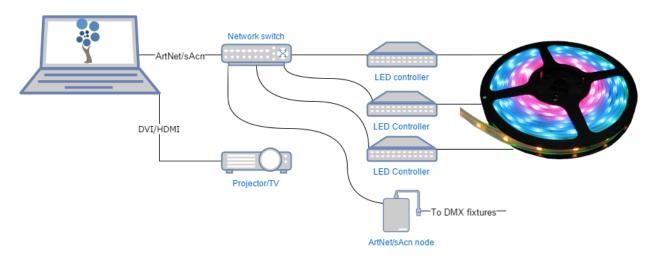
The next step is to get LED strips and DMX fixtures. Since there are many LED protocols out there, you need to make sure your LED controller fits with your LEDs. Common protocols for RGB LEDs are WS2811 and WS2812/B. For more information about getting compatible LEDs, contact your Enttec representative. Here's the Enttec Pixelator that can be used to control the Phero and Enttec LED tapes:
