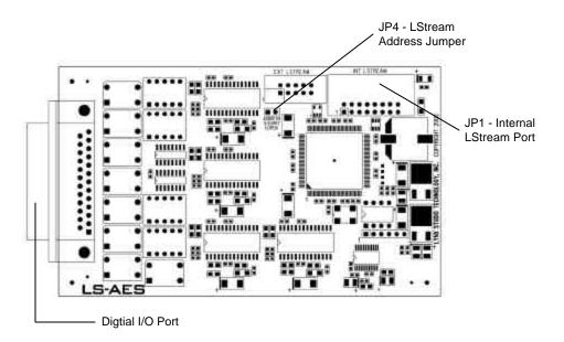
Connect the included breakout cable to the bracket-mounted Digital I/O Port connector on the LS-AES. The XLR connectors on the cable connect directly to equipment with AES/EBU ports. For S/PDIF coaxial connections, use Lynx XLR to RCA S/PDIF adapters (CBL-XFDRM18 and CBL-XMDRM18). The following table shows the audio signal channels associated with each cable connector.
