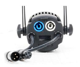
The Saber Spot WW is a compact Pinspot with a 15-Watt warm white LED. Features DMX-512, flicker-free operation, strobing, electronic dimming and has a 4-Button DMX display system on the rear panel. Its built-in ACL lens produces a razor sharp 4-degree beam angle.
