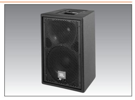
distortion resulting from turbulence. The horn design with its large mouth delivers smooth, natural reproduction - especially in the critical mid-range. A 16 gauge, steel grill protects the ten inch JBL woofer. Designed for portable applications in live performance, music playback, and reinforcement of speech, the MP410 will deliver excellent performance by itself or as a satellite over subwoofers such as the MP418S and MP418SP.
