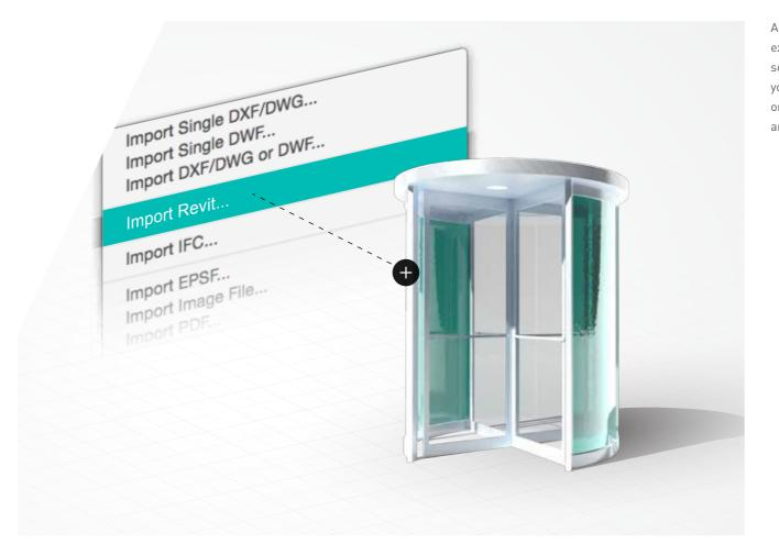
Architects and landscape professionals must be prepared to exchange data with other BIM collaborators. In Vectorworks software, you can now import Revit files directly, allowing you to manipulate manufacturer-specific objects from Revit or to collaborate more effectively with other designers and contractors throughout the lifecycle of your project.
