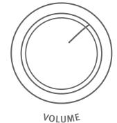
The VOLUME potentiometer is motorized and can be remotely controlled (see page 14).
