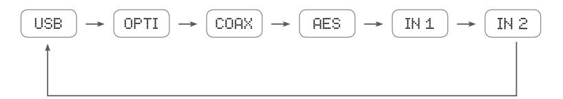
When a digital source is selected, its name is displayed for about two seconds (USB, OPTI, COAX, AES). After that the first letter of the name appears together with the sample rate which is automatically detected by the Director (e.g. USB4, O192). See table on the next page.
