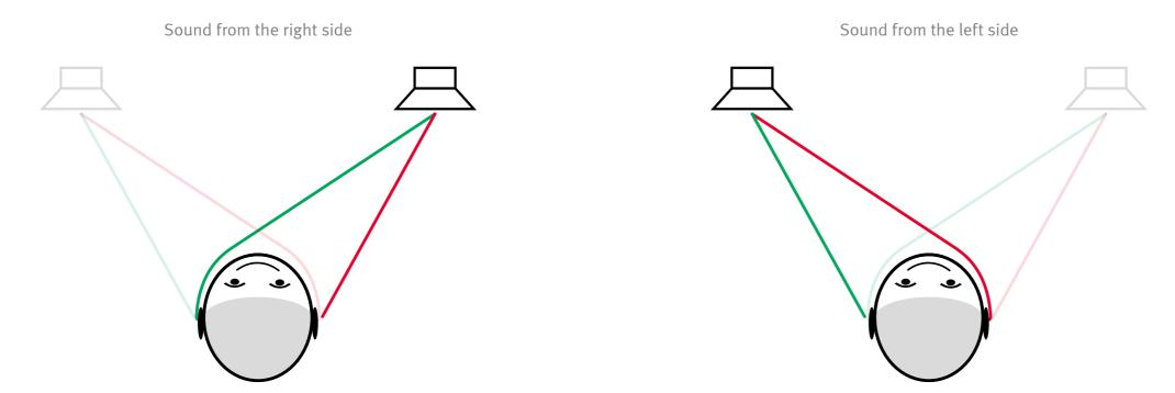
It arrives later because the signal travels a distance of approx. 340 meters per second and the distance from the right speaker to the left ear is longer than it is to the right ear. It is quieter and does not deliver the full frequency range, because the signal of the right speaker does not directly arrive at the left ear but is partially reflected and absorbed by the head.
