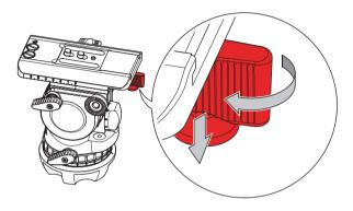
**4.** The camera plate or camera will be released from the sliding balance plate.
