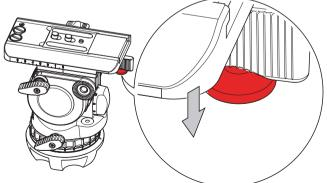
**3.** With the safety button held down, move the locking lever as far as possible to the left.
