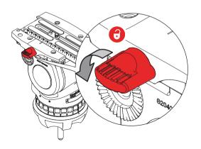
3. Push the safety lock (1) and release the plate (2).
