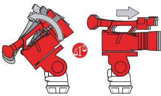
**(c)** If the payload tilts forwards (points down), slide it towards the rear of the fluid head. Re-lock the sliding balance plate.
