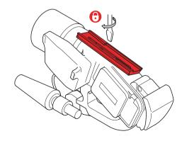
**5.** Place the camera plate into the dovetail and lower into place. It will lock automatically and the lock lever will click audibly back into its initial position.
