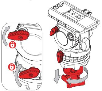
Move the head so that the level bubble is central. Tighten the tie down, release the horizontal brake and check the level bubble remains central.
