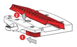
4. Attach the camera plate to the camera around its centre of gravity, observe the arrow on the plate indicating the direction of the arrow. Additional screws are stored in the sliding balance plate assembly.
