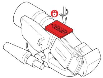
**6.** Mount the camera plate and camera onto the sliding balance plate. It will lock automatically and the lock lever will click audibly back into its initial position.
