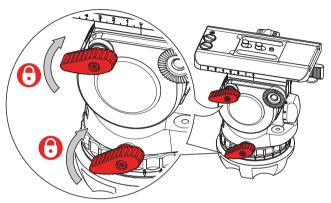
2. Hold the camera plate or camera with one hand. Grasp the locking lever with your thumb and index finger and pull down the safety button.
