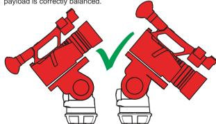
If the payload continues to move upwards when released, the balance is set too high. Lower the balance adjuster setting by one increment and retest.
