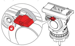
**(b)** If the payload tilts backwards (points up), slide it towards the front of the fluid head. Re-lock the sliding balance plate.
