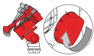
4. If the payload continues to move backwards when released, the balance is set too low. Raise the balance adjuster setting by one increment and retest.
