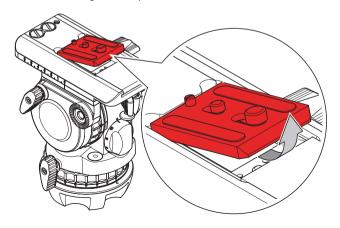
**5.** Attach the camera plate to the camera around its centre of gravity. Additional screws are stored in the sliding balance plate assembly.
