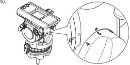
2. Tilt the payload approximately 30° in both directions and release it. If the payload stays in the same position when released, the payload is correctly balanced.
