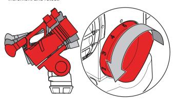
Tilt the payload through positive and negative angles of travel, checking that the payload remains at any angle of tilt unsupported.
