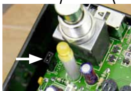
OUT-B jumper in the default position
