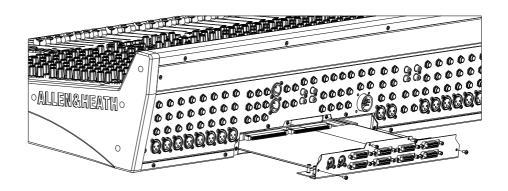
Slide the module into the housing and push firmly to insert the module connectors into the console connector sockets.
