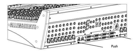
To remove the module for any reason, the easiest way is to unscrew and remove the fixing screws at each end of the panel then use the D Sub cable connectors to gently pull out the module. A small side to side rocking action will help to displace the circuit board connectors from the internal mother-board.
