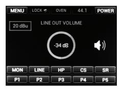
Enter the Line Out menu to adjust the output volume level.
