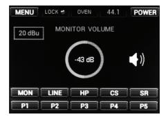
Enter the Monitor menu to adjust the Monitor volume level from the screen or the main Volume Knob.
