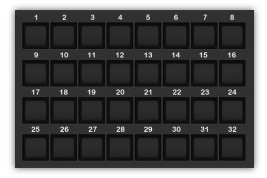
These 32 buttons can be used to call lighting effects, scenes, colors, etc. If your lighting software does not support the **MIDICON-2™** as plug and play, you will have to link each button to a function using the setup menu in your software. Refer to your software manual for instructions, as this will be different for each program.
