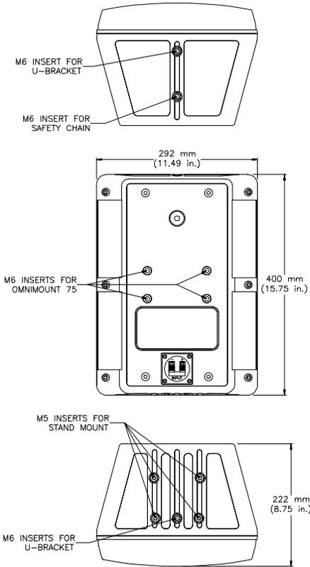
Figure 8— Sx80 enclosure with Sx80MB wall/ceiling mounting bracket.
