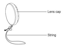
2) Thread the other end of the string through the hole on the bottom of the projector.
