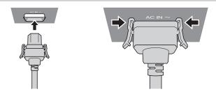
1) Check the shapes of the <AC IN> terminal on the back of the projector body and the power cord connector and insert the plug completely in the correct direction (until you hear the side tabs click in place).
