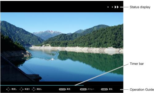
Display example (10 speed) fast-forward during playback
