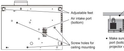
Make sure the air flow into the air intake port (bottom), failure to do so may cause the projector cannot work.
