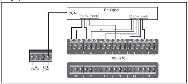
Per diagram when the fire signal is received connect so that the proper channel is activated to send emergency broadcast.
