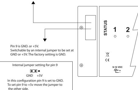
The Factory setting is for pin 9 set to GND making the logic 0 when the CONTESTANT led is ON, and logic 1 when the led is off. When the internal jumper is set to +5V for pin 9 the logic is then reversed (led on is logic 1, led off is logic 0).
