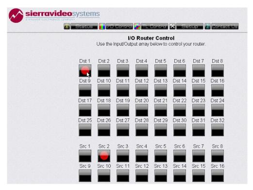
To switch the router, select (left mouse click) on a destination, the button will turn red. The current status will be indicated by the current source button will turn red.
