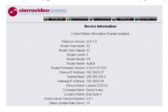
To setup IP address parameters, select "Setup".
