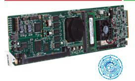
Alternate Base Models 9374-EM Quad-Stream SDI - AES - MADI Embedder 9374-DE Quad-Stream SDI - AES - MADI De-Embedder The 9374 offers our most comprehensive solution for digital audio transport conversion and embedding/de-embedding. A full unrestricted audio crosspoint provides channel routing between any channels on up to four SDI streams, discrete AES-3id, and AES-10 MADI interfaces.
