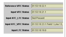
If Audio/RS-485 LTC is being received on selected LTC Input source, the timecode running count is displayed.
