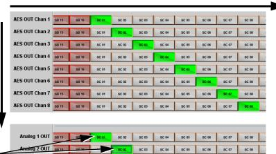
Analog 1/2 OUT radio buttons provide direct routing of selected channels to the card stereo analog audio monitor outputs. Selecting another monitor input clears any prior selection. (Selections made here are reflected on the Input Meters tab, with changes made on either tab correspondingly reflected on the other.)
