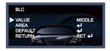
→ HSBLC (Highlight Suppression Back Light Compensation): When there is a car head light turned on at the entrance of the gas station or in some place in the parking lot, the numbers of the car plate can be recognized by blocking only the light from the car headlight. The area is set up specifically so you can recognize the car plate numbers by blocking out the strong light.
