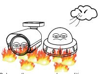
Only use the camera under conditions where temperatures are between -4°F and +140°F. Be especially careful to provide ventilation when operating under high temperatures.
