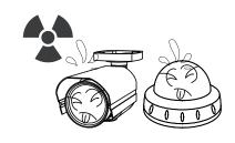
If exposed to radioactivity the CCD will fail.
