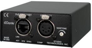
channels can be interconnected (routed) with other devices using the Dante Controller software application. The Dante transmitter and receiver channels are limited to supporting four Dante flows, two in each direction. The digital audio's bit depth is 24 with a sampling rate of 48 kHz.
