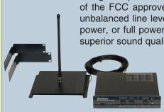
Designed specifically to help people with partial hearing loss, the TX-37A is field tunable to 37 of the FCC approved channels for ALS. Its universal input accepts mic level, balanced and unbalanced line levels, and speaker level. Signal strength is adjustable to quarter power, half power, or full power. Audio processing eliminates clipping and over-modulation while providing superior sound quality, increased intelligibility, and dynamics control. #910-402-010
