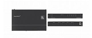
The VM-4UHD is a 4K UHD 1:4 distributor for HDMI signals. It takes one HDMI input, equalizes and reclocks the signal and distributes it to four identical outputs. The VM-4UHD distributes signals having resolutions up to 4K@60 UHD (4:2:0), WUXGA and 1080p.
