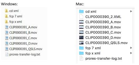
Each camera or video feed input has its own .mov file designated A / B / C / D as shown above – the \_QSLS movie file is generated when the option for Live Switch or Quad Split is enabled on the Odyssey / Apollo. If HDMI is one of the video feeds, then it will in be the \_A file.
