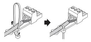
Trim off the extra portion of the cable tie as necessary.
