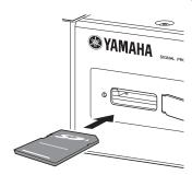
When the SD memory card has been correctly recognized, the [SD/ACT] indicator (page 9) will light. The [SD/ACT] indicator will flash while the card is being accessed.
