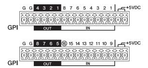
The MRX7-D provides 16 input ports and 8 output ports.
