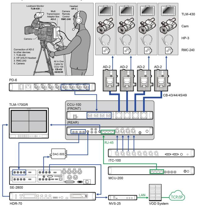
Communication between AD-2 (S/P/J) and CCU-100 is bidirectional. The signals in each direction are listed below:
